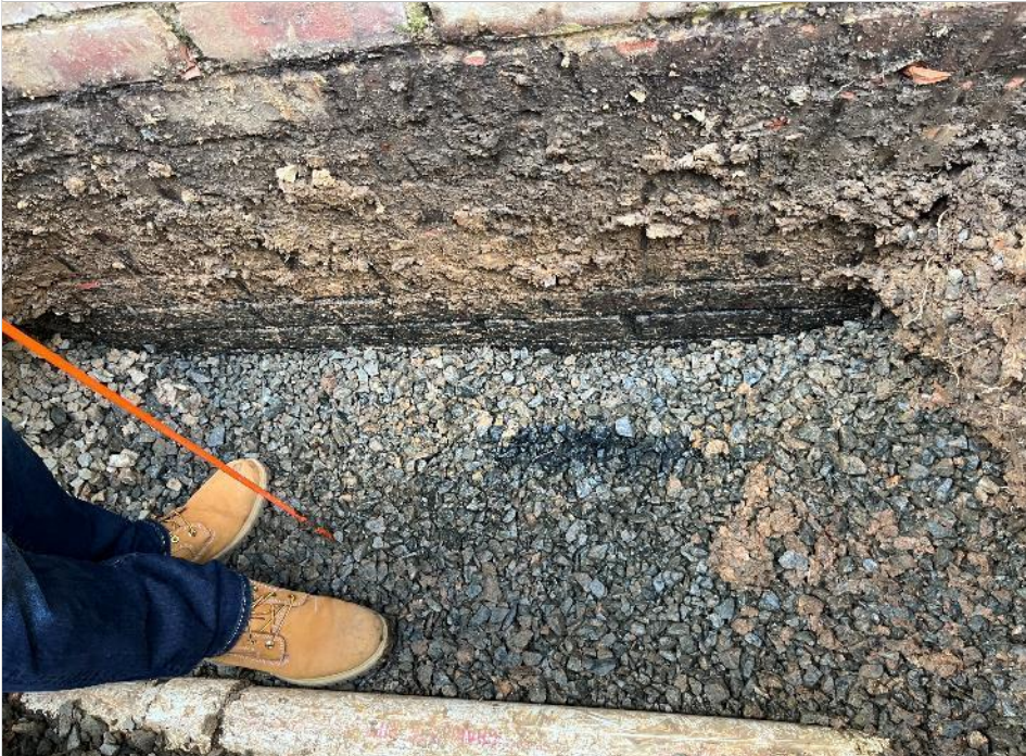
Photo 10 – Test Pit #4: Thin applied coating installed on brick within test pit. Gravel encountered at bottom of test pit.
