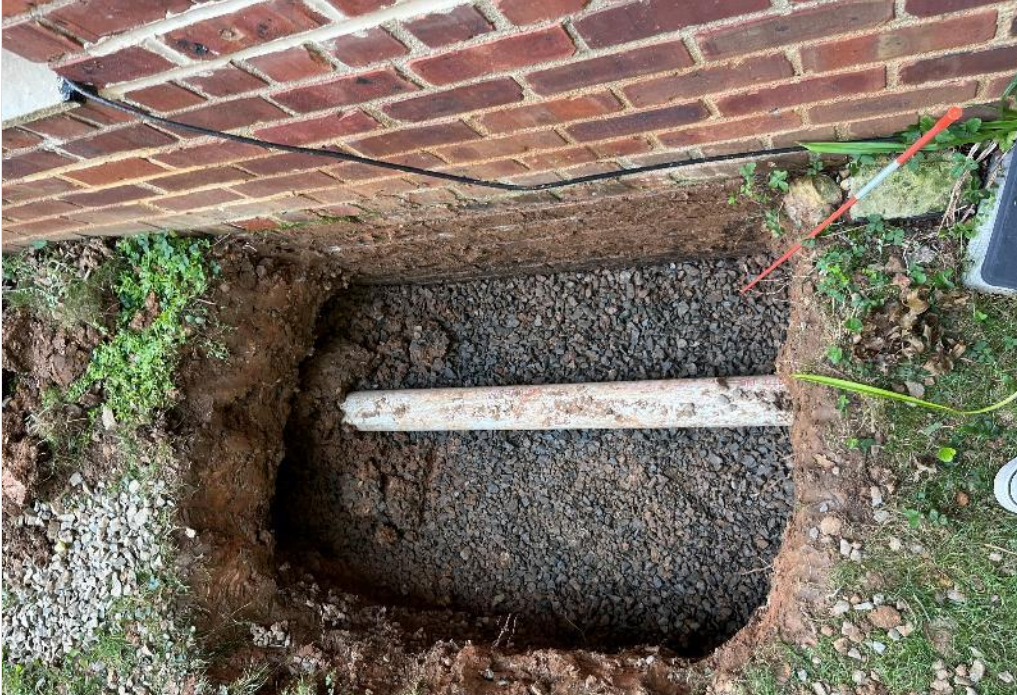
Photo 8 – Test Pit #3: Gravel encountered at bottom of test pit. Downspout attached to horizontal PVC pipe in test pit.
