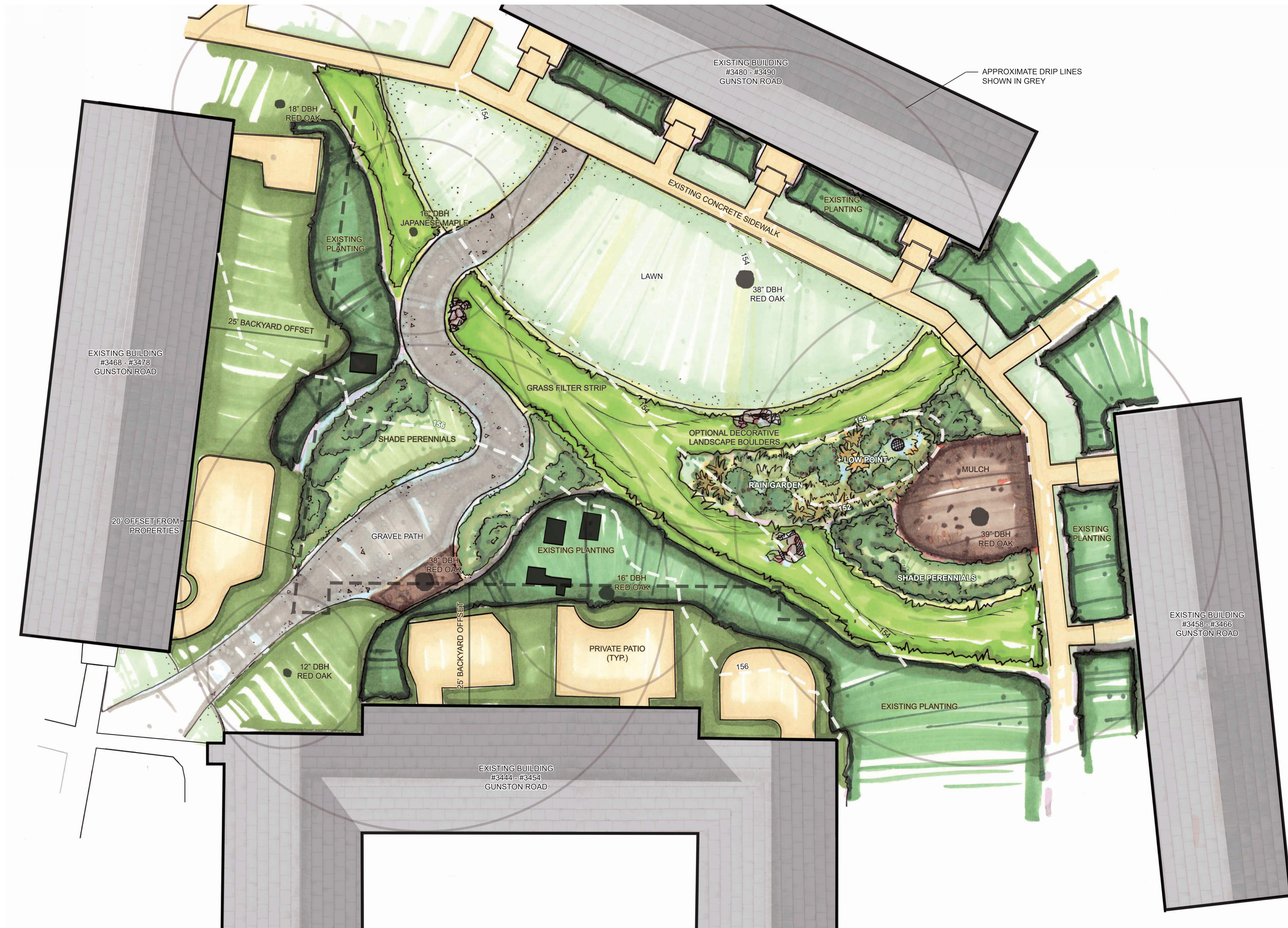
Grass Filter Strip As stormwater moves through grass, it slows down and sediment is filtered out. Putting swaths of Pennsylvania Sedge - a shade tolerant and vigorously growing ornamental grass - throughout this site would quickly stabilize the soil, absorb runoff and sediment, and create a peaceful river of flowing grass fronds. By mowing this a few times a year, a shorter grass can be achieved that is less likely to harbor small mammals.
